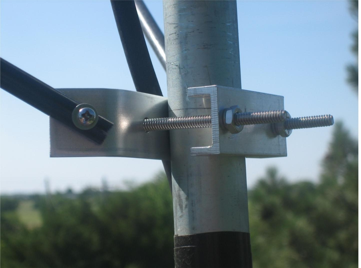
Note: The bolts mounting the fiberglass support rods (both ends) have been replaced with clevis pins.
